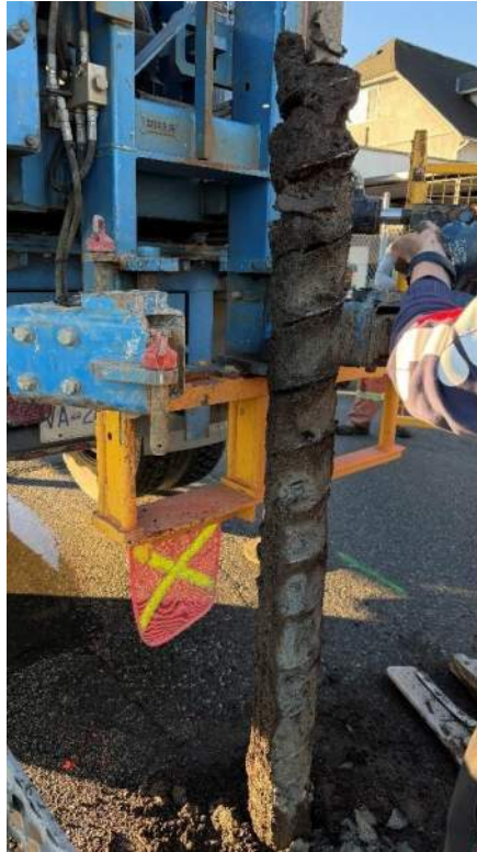
Photograph No. 5 Soil stratigraphy at AH26-01 from 5'-10' (1.5 – 3.0 mbgs).
