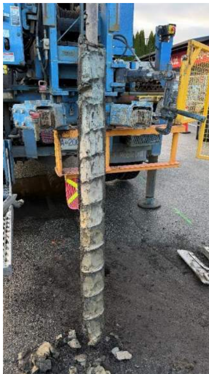
Photograph No. 6 Soil stratigraphy at AH26-01 from 10'-15' (3.0 – 4.5 mbgs).
