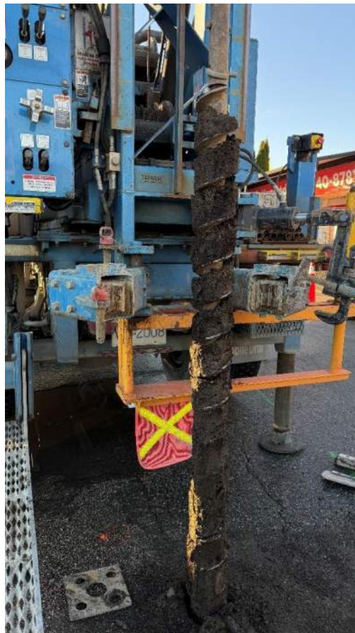
Photograph No. 4 Soil stratigraphy at AH26-01 from 0'-5' (0 – 1.5 mbgs).
