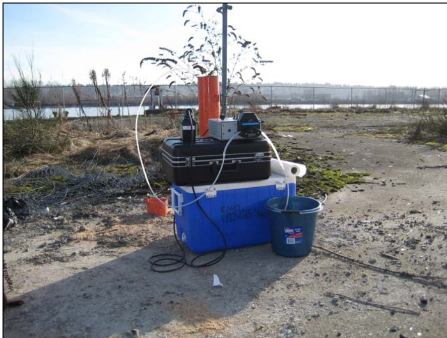
Photograph 6: Showing a groundwater monitoring well being purged prior to sampling
